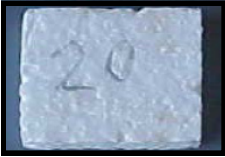
Termite attack on EPS treated with Imidacloprid
